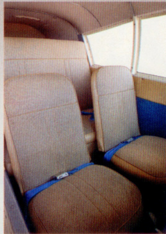
Small clues in the interior tell of an early Cherokee. The door handle (far left) and low seatbacks (left) were kept for a number of model years later, but the unique latch (below left) and overhead trim crank (below) were dropped soon after.
